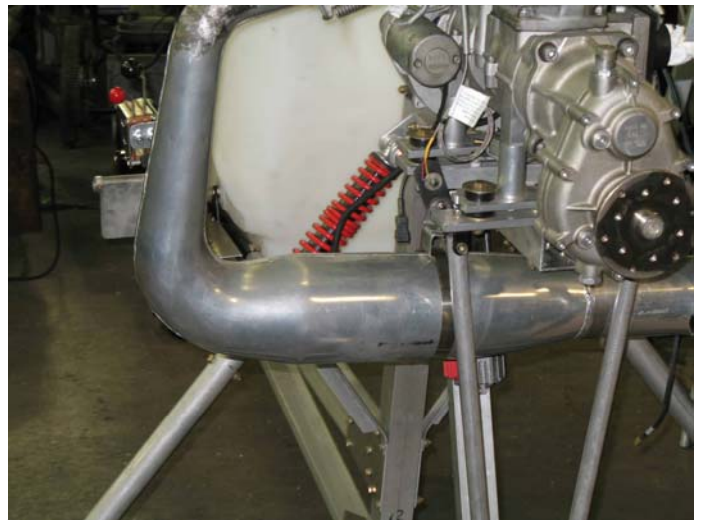
Adam's MZ 202 engine and muffler were mounted over the last few weeks during the Wednesday night builds.
